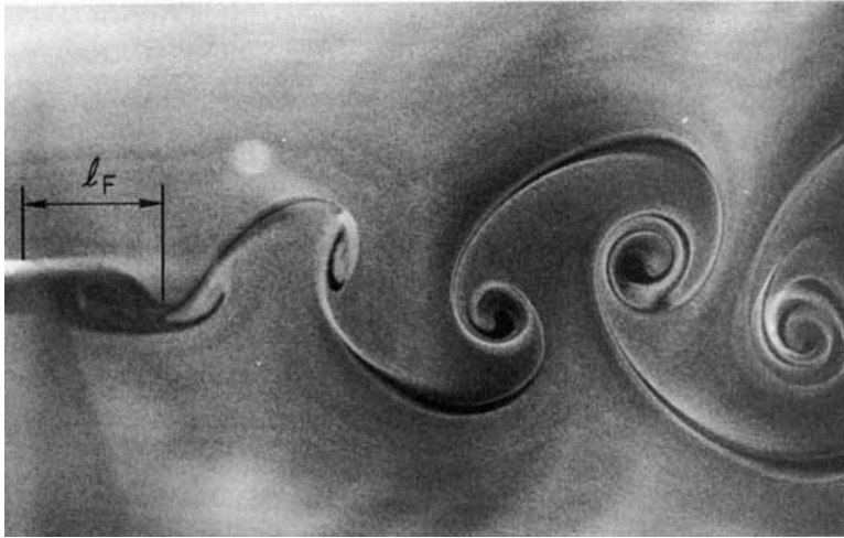
FIGURE 1. Flow visualization of the vortex formation and near-wake flow for a circular cylinder at a Reynolds number Re = 200 . The wake was visualized by introducing a sheet of aerosol particles into the wind tunnel contraction section (Griffin & Votaw 1972; Griffin & Ramberg 1974). The cylinder is oscillating at an amplitude of a/d = 0.15 and a frequency f = 0.85f_{so} ( f_{so} is the Strouhal frequency).
